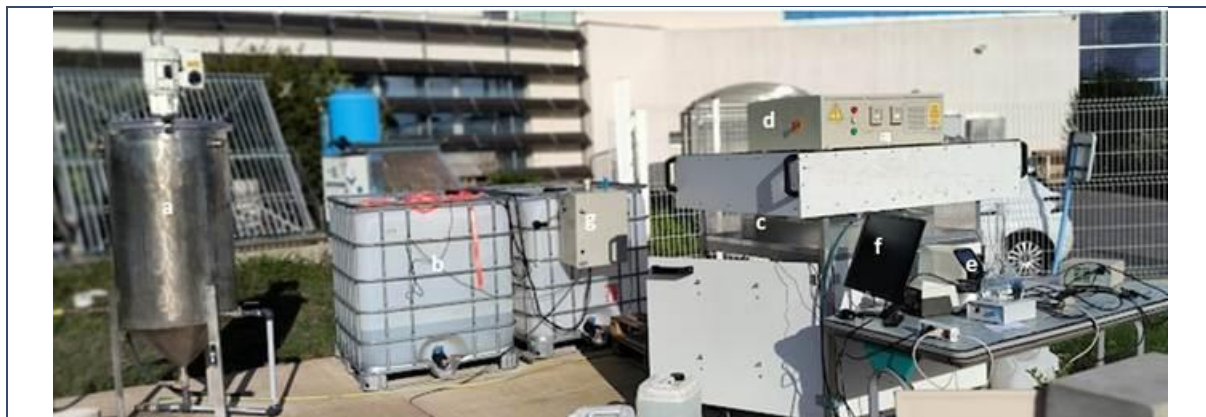
Figure 8. View of the entire installation for solar experiments consisting of (a) the network water supply tank, (b) the treated water collection tank, (c) the basin-type photoreactor, (d) the artificial lighting system (LED panel and power supply), (e) the pollutant supply system (peristaltic pump), (f) the supply control panel, valves, agitation and lighting and (g) the sensors and power supply.
