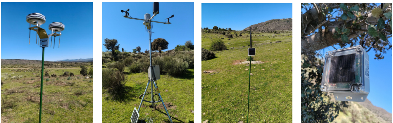
A network of low-cost environmental sensors (weather, soil and air quality) connected via LoRaWAN for real-time monitoring.
