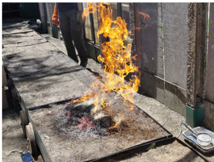
Photographs of the two types of experimental burning carried out in the ICIFOR-INIA (CSIC) wind tunnel. Left: Arbutus unedo (strawberry tree), freshly collected vegetation. High humidity with smoke predominating over flame. Right: Pinus pinea (stone pine), vegetation collected previously and prepared. Low humidity, with high flames predominating.
