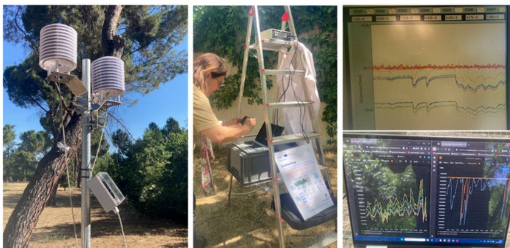
Electronic modules fitted with microsensors from the IMB-CNM (CSIC) installed at INIA (CSIC) to monitor the burning tests carried out in the wind tunnel.
