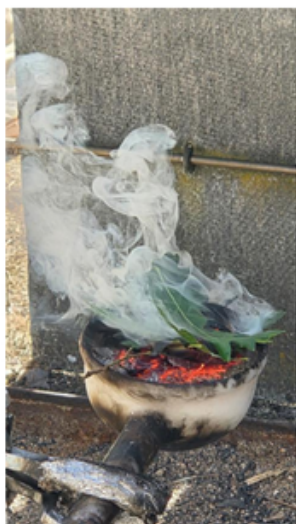
Photographs of the two types of experimental burning carried out in the ICIFOR-INIA (CSIC) wind tunnel. Left: Arbutus unedo (strawberry tree), freshly collected vegetation. High humidity with smoke predominating over flame. Right: Pinus pinea (stone pine), vegetation collected previously and prepared. Low humidity, with high flames predominating.
