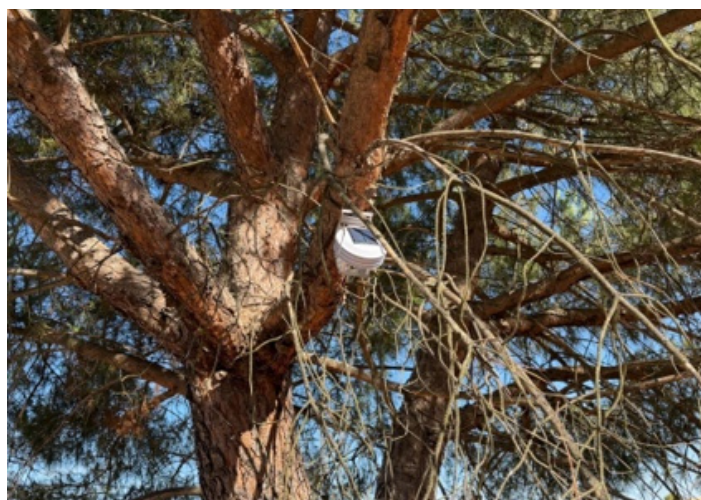
MOX, EC and PM sensor nodes and a LoRa router deployed near the Las Vaguadas neighbourhood (Badajoz).
