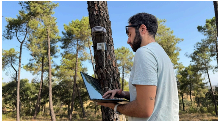
On-site firmware update of a sensor node to prevent data transmission errors.
