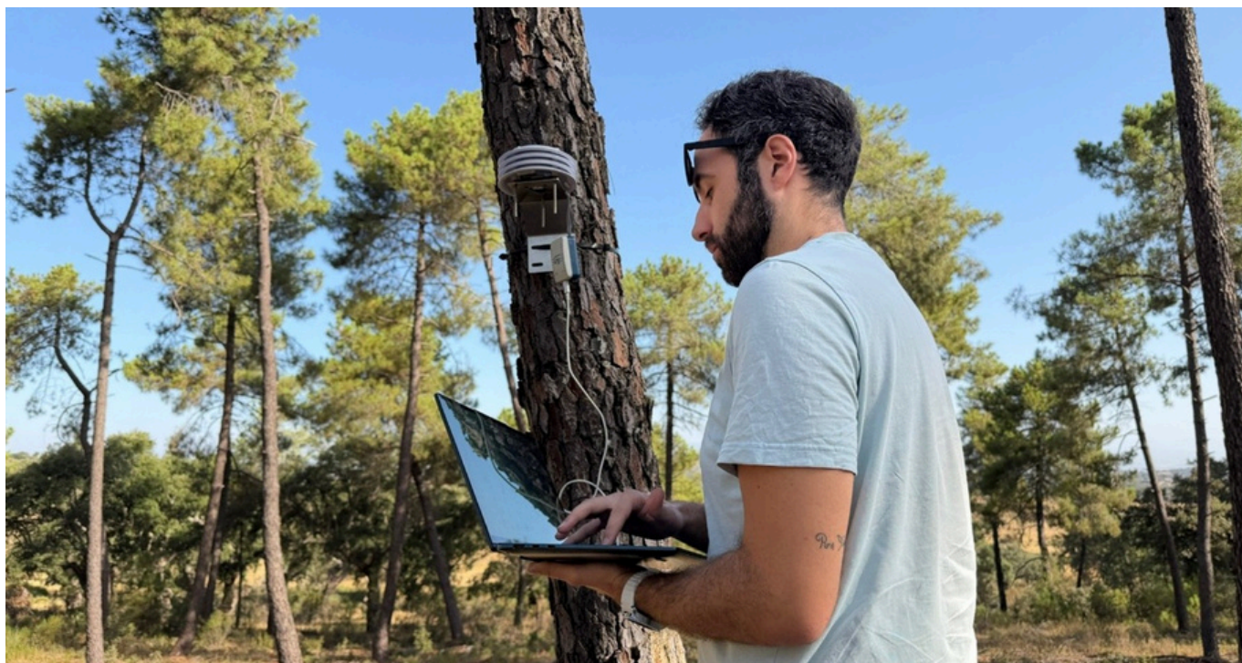
Ángel López (UEx) updates the firmware of a SenForFire sensor node in the pilot areas of Cáceres.
